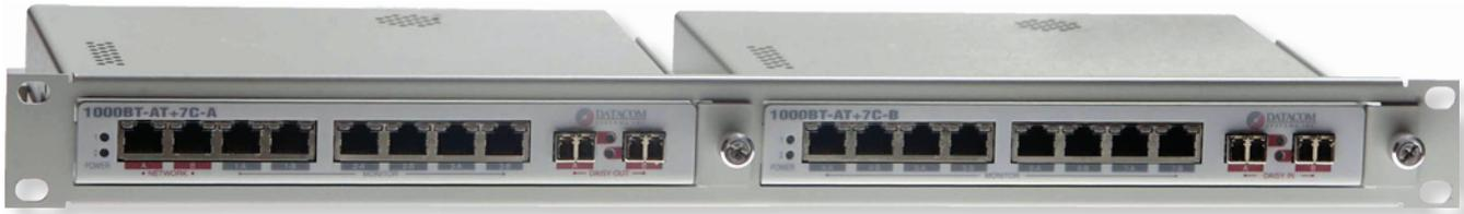
The Copper Gigabit Regeneration Tap provides easy 24 x 7 access to your Gigabit Ethernet segments. Three devices, such as intrusion detection systems, protocol analyzers, or probes can access the same segment at a single point, eliminating contention for network links. With redundant power supply and fault tolerant design, network performance and integrity will not be affected by power loss.
