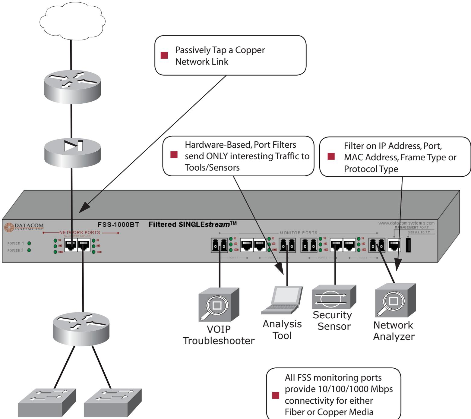
■ Taps provide improved visibility over SPAN ports
