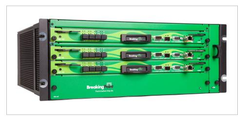
BreakingPoint FireStorm is used to evaluate, size, and configure IT infrastructures to perform optimally and securely while under load from millions of users, hundreds of applications, and thousands of cyber attacks. This all-in-one cyber security system pinpoints previously impossible-to-detect weaknesses and vulnerabilities in networks, network devices, and data centers before they can adversely affect IT operations.
